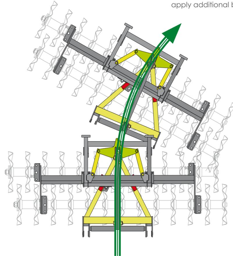
Through the trapezium guide the rollers are directed automatically into the direction of motion.
