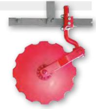
The disc coulter is adjustable in all directions and therefore is able to get adapted to every given situation.
