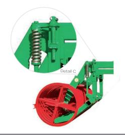
ig(i) Avoid comering on all types of rollers as the bearings can be damaged
