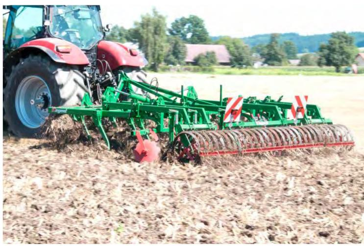
The Tukan DSG in the 4 beams version is suitable for middle to heavy soils at a working depth of approximately 10 to 30 cm.
