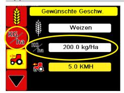
In the next window, you can set the desired seed rate. To do this, select the KG / ha symbol and enter the desired amount. The seed rate can be changed later in the main display, e.g. to to be able to react quickly to changing soil conditions.
