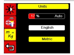
After activating the window, the desired unit of measurement can be activated using the rotary button.
