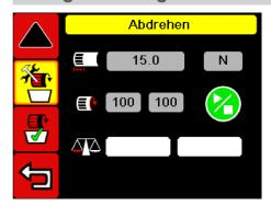
The dosing unit must be adapt fot the calibration test before before you start with the sample. The display shows the value to which you must set the seed wheel. In this case the value 15 should be set. The fan flap must be in position N.
