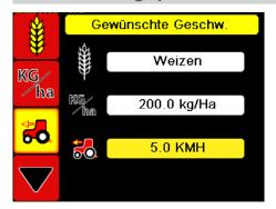
Now the expected driving speed is set.With the double disc and hydraulic coulter pressure monitoring, this speed will be between 8 and  $15\,\mathrm{km}$  / h
