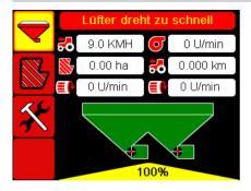
In order to prevent damage to the blower, the speed must be reduced as quickly as possible. The maximum speed is 3000 rpm.
